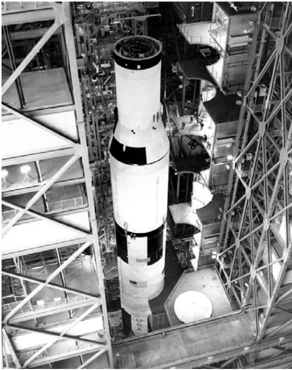
Figure 2- Saturn 505, AS-505, ready for the Apollo 10 payload in high bay 2 of the Vertical Assembly Building at Kennedy
