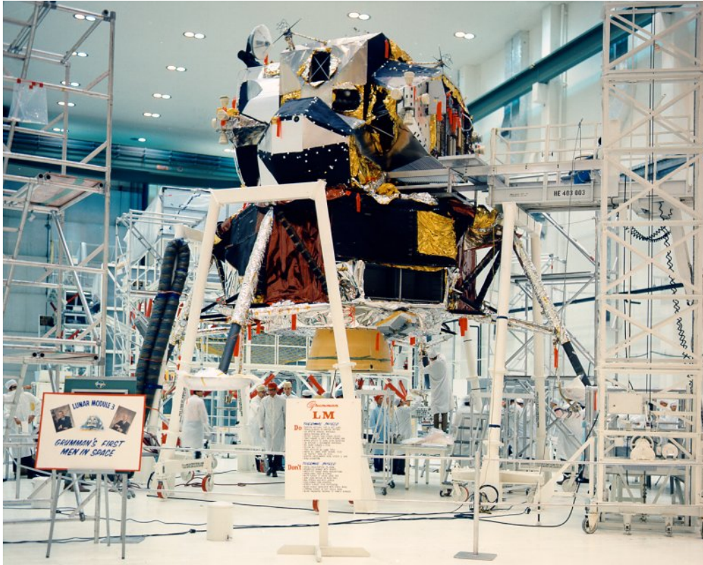
Figure 3 – LM-3 at Kennedy Space Center’s MSOB prior to transfer to the Vertical Assembly building. Note the support struts preventing the crushing effects of Earth’s gravity and the segmentation between the Ascent and Descent stages. The large descent engine bell is shown toward the bottom center in yellow.
