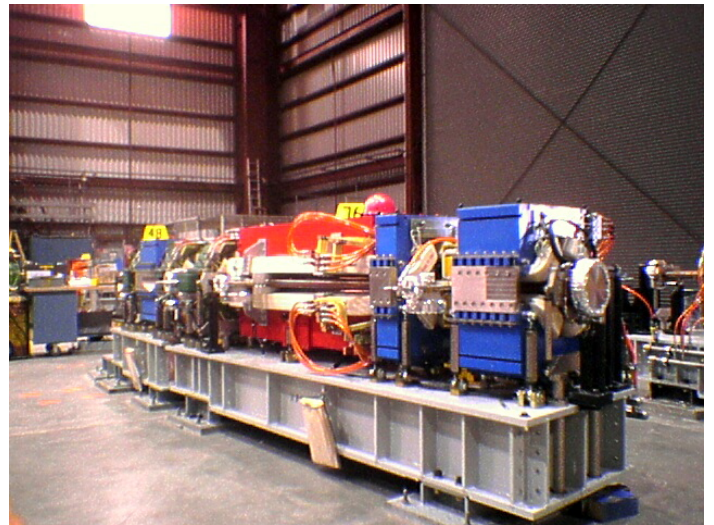
These units generate magnetic fields that can steer subatomic particles and direct them to collide with one another.
