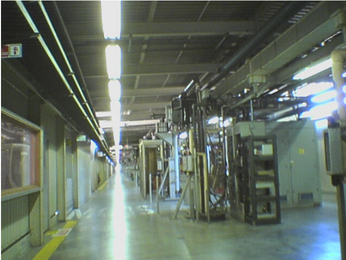
A view down the accelerator tunnel. The main accelerator is 25 feet underground. The machinery here on the surface are microwave generators that accelerate subatomic particles.
